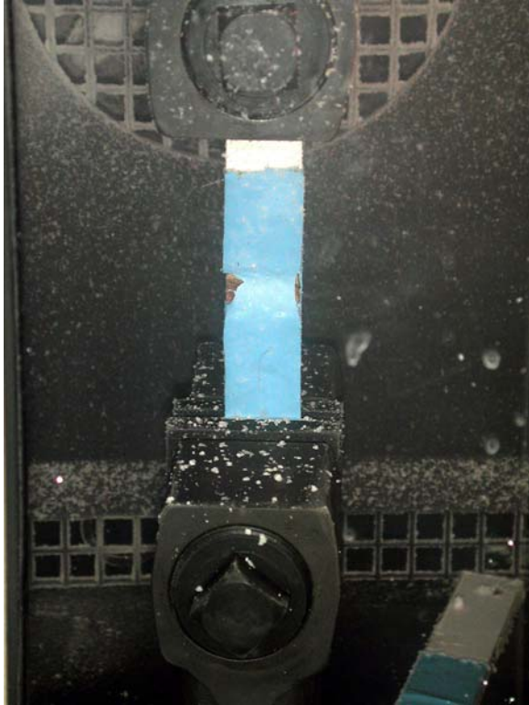
Figure 5. Specimen failing at -30°C
