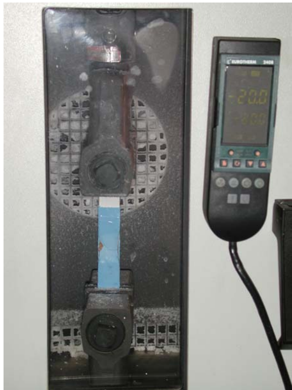
Figure 6. Specimen failing at -20°C
