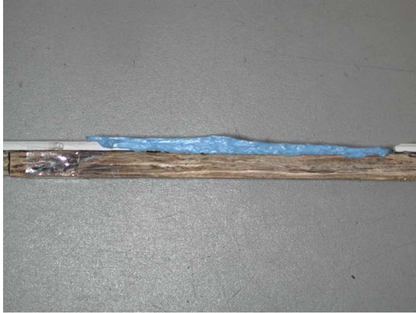
Figure 4. Close-up of overlap between PVC and OSB
